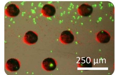
Magnetic pillars trapping red particles in a microfluidic channel with non-magnetic cells (in green).
