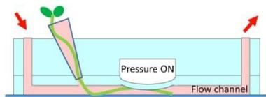
hydroponic chips for in-chip growth and microscopic study of *Arabidopsis thaliana* roots. The objective is to design microfluidic
